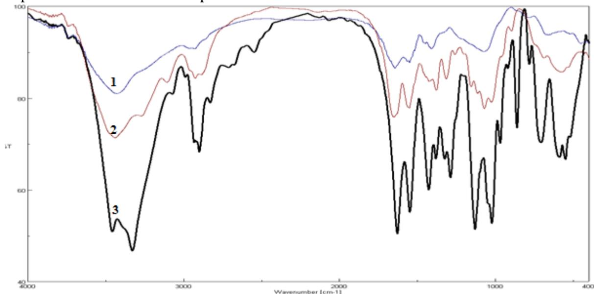
Fig. 5. FTIR spectrum of (1) COS, (2) chitin and (3) N-acetyl glucosamine.
