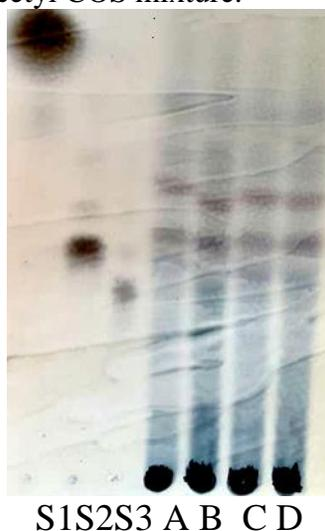
**Fig. 4.** TLC plate of SPB hydrolyzate in which S1, S2, S3 are N-acetyl glucosamine, N-acetyl chitopentose and N-acetyl chitohexose standard respectively and A, B, C, D are the initial, after autoclaving, after filtration and ethanol precipitated hydrolyzates.
