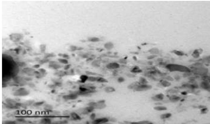
Fig.1. Transmission electron microscopy (TEM) image of copper oxide nanoparticles.
