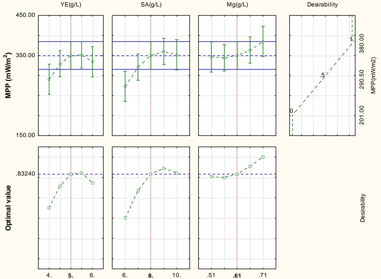
**Fig.3: Desirability and prediction profile for the MPP in Box-Behnken design.**
