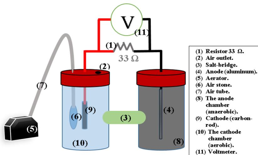
Fig. 1: A schematic diagram of the constructed double-chambered microbial fuel cell.
