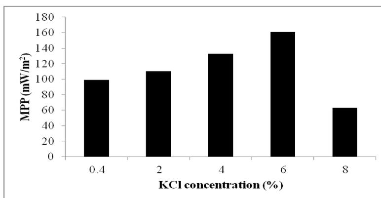
Fig. 2: Effect of different potassium chloride concentrations in salt-bridge of the MFC.
