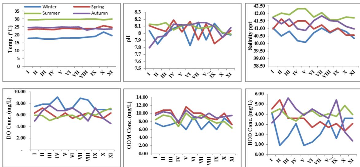
Fig. 3: Temp. (°C), pH, Salinity (%), DO, OOM and BOD (mg/l) fluctuations of water samples collected from the study area during 2017.
