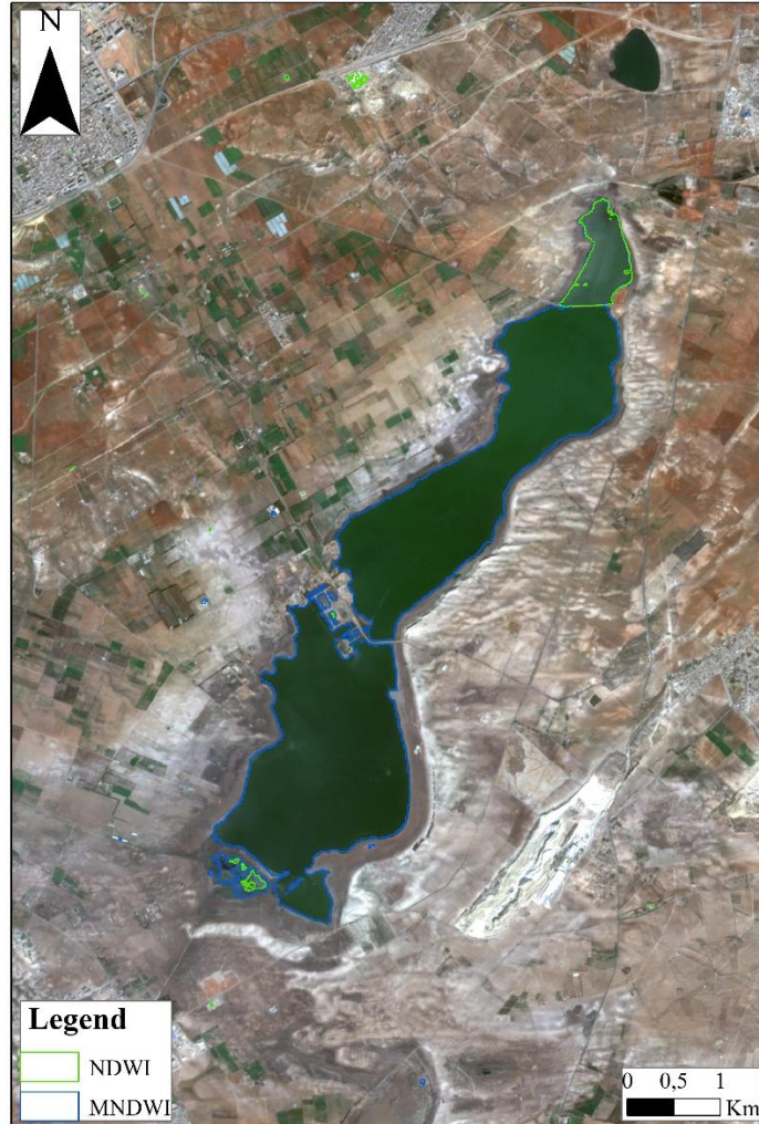
Fig. 9. Illustrative images of Telamine Lake (21/02/2024); True color based on bands B4, B3, B2, Bleu color: MNDWI based on bands B3 and B11, Green color: NDWI based on bands B3 and B8
