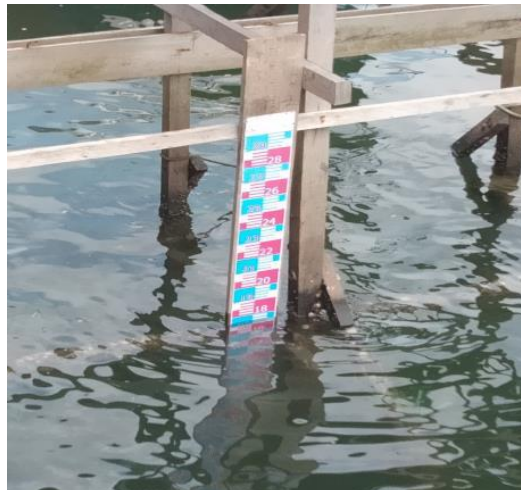
Fig. 3. Tide staff installation for measuring tidal fluctuations
