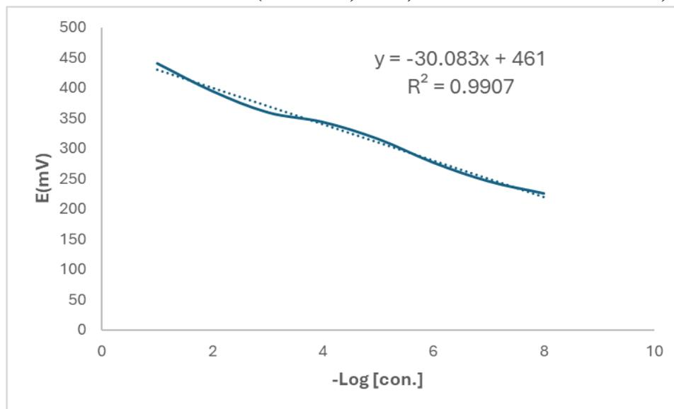
**Fig. 9.** Calibration curve of modified carbon paste electrode
