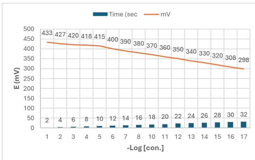
**Fig. 8.** Response time modified carbon paste electrode
