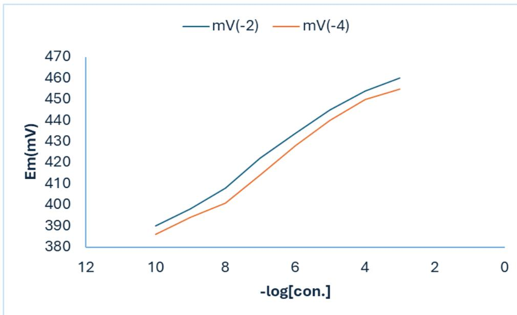
**Fig. 6.** pH effect on modified carbon paste electrode
