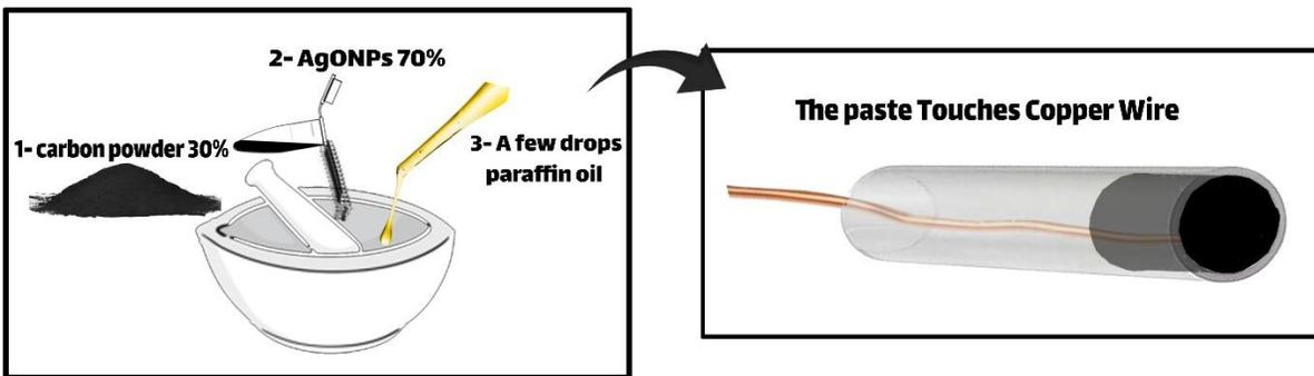
**Fig. 2.** The electrode preparation
