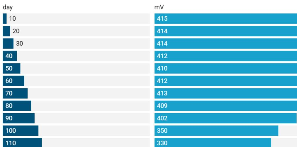
**Fig. 10.** Lifetime of modified carbon paste electrode
