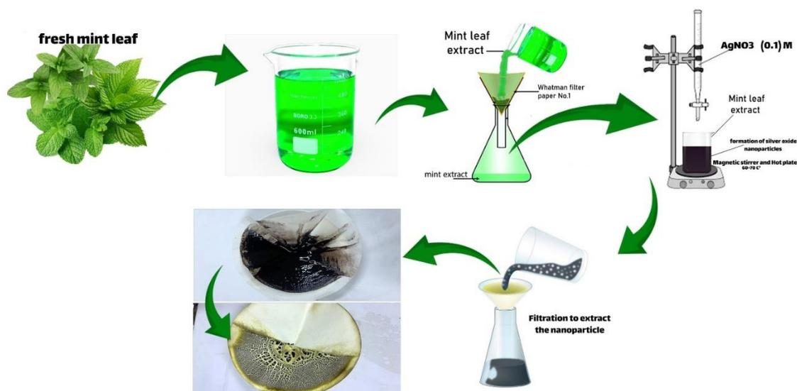
**Fig. 1.** Plant extract and silver nanoparticles preparation
