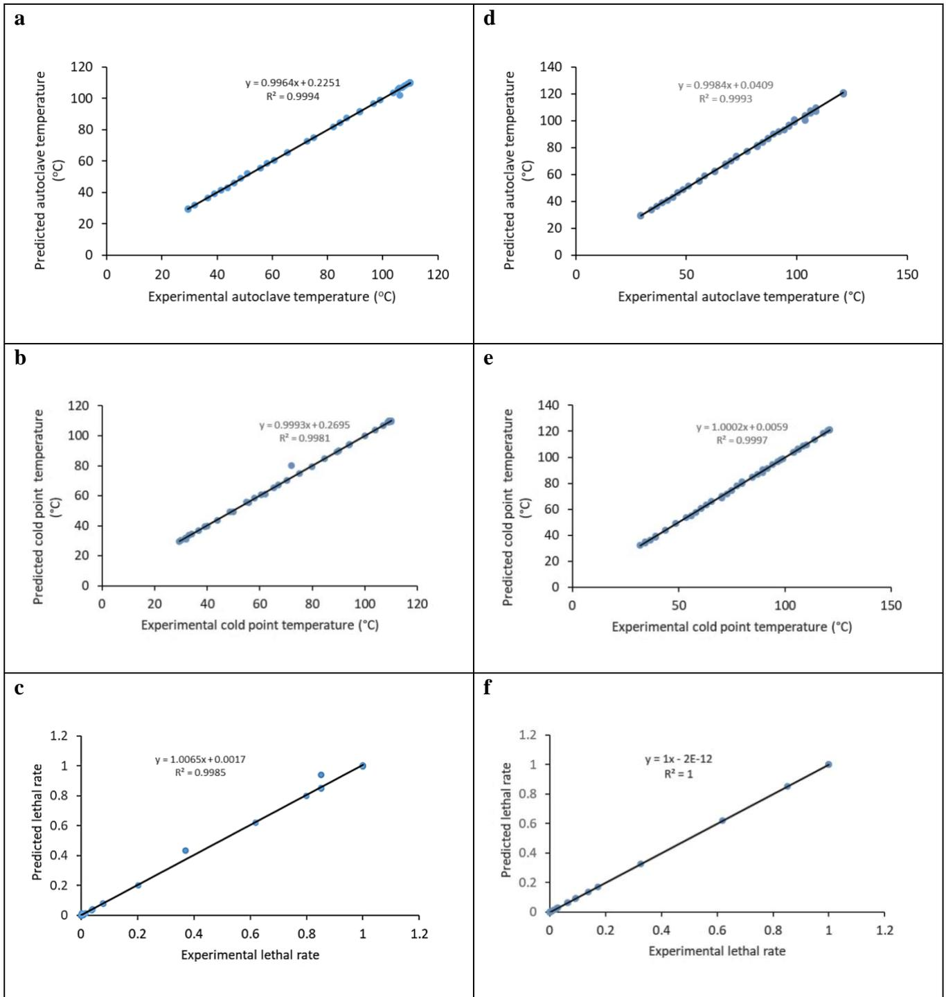
**Fig. 7.** Correlation coefficient between experimental and predicted of autoclave temperature, cold point temperature, and lethal rate at temperature of 110°C (a, b, c) and 121°C (d, e, f), respectively.
