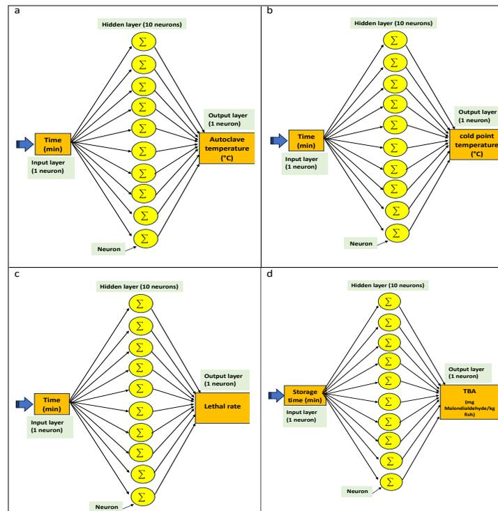
**Fig. 1.** The feedforward neural network with multilayers: (a) Prediction of autoclave temperature, (b) cold point temperature, (c) Lethal rate, and (d) TBA
