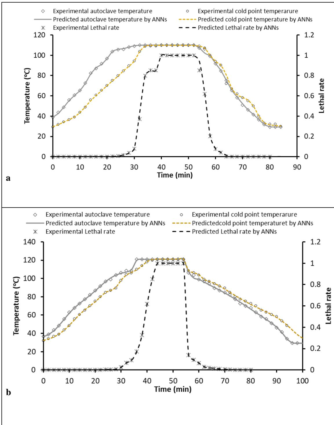
Fig. 2. Experimental and predicted of heat penetration curve of sterilized canned fish by autoclave at temperature of a: 110 °C, and b: 121°C
