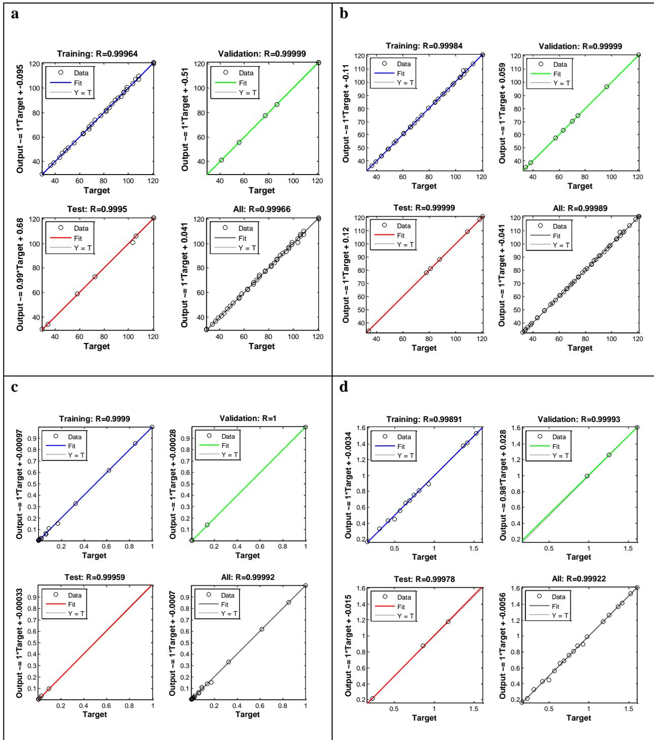
**Fig. 5.** ANN performance at 121 °C temperature via correlation coefficients (R). (a) Autoclave temperature, (b) cold point temperature, (d) lethal rate for training, validation, testing. The target data are experimental and the output data are the predicted
