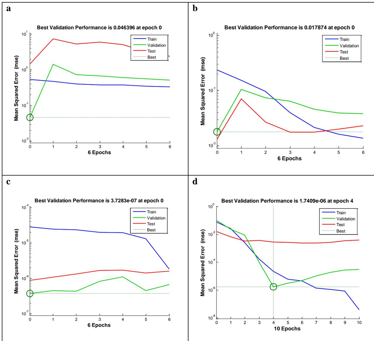
**Fig. 6.** ANN performance at 121°C temperature by mean square error (MSE). (a) Autoclave temperature, (b) cold point temperature, (c) lethal rate, and (d) TBA
