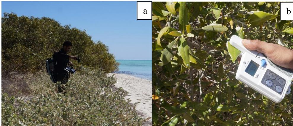
**Fig. 2.** Measurement on field with different instruments; **a**, Spectroradiometer, **b**, Chlorophyll meter
