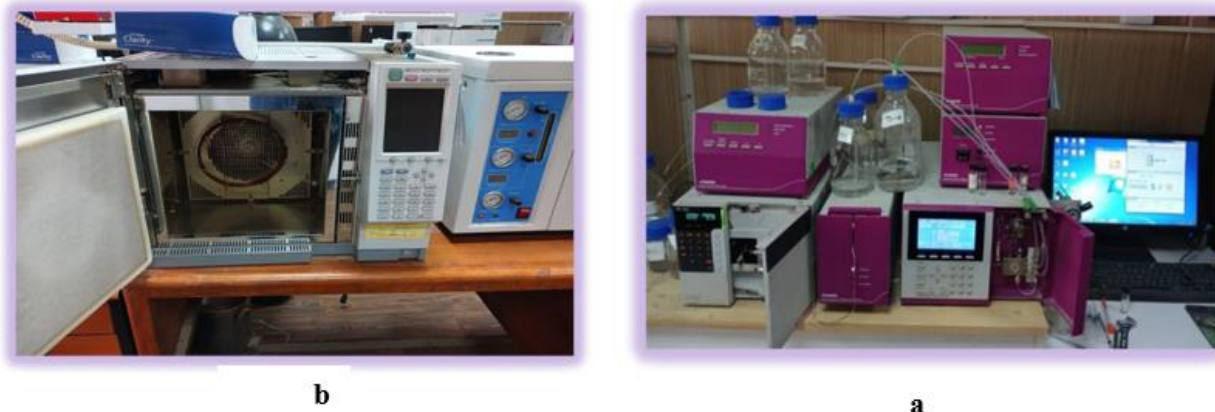
Pic. 4. (a) HPLC device for amino acid analysis; (b) GC device for analysis of fatty acids in shrimp Metapenaeus affinis
