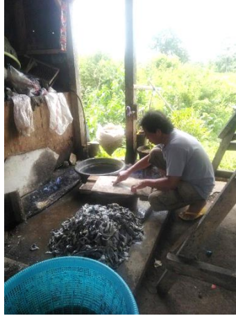
Fig. 4. Skiving process applied to the fish skin
