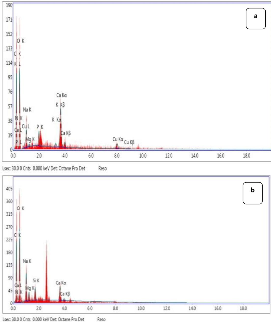
**Fig. 3.** EDAX of: **(a)** Crab chitosan and **(b)** Crab chitosan nanoparticles
