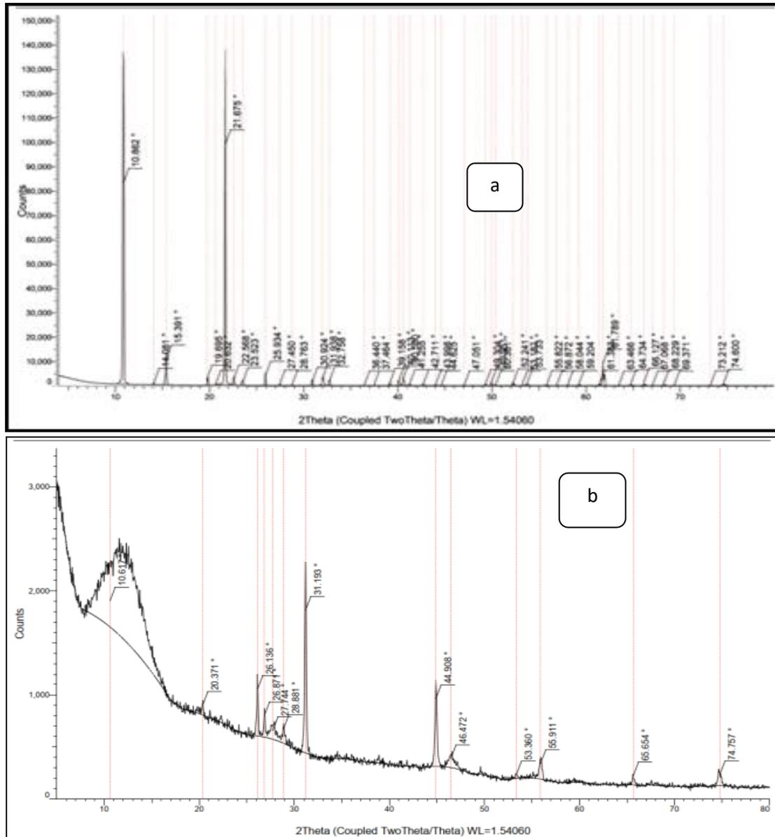
**Fig. 2.** X-ray diffraction patterns of: (a) Crab chitosan and (b) Crab chitosan nanoparticles
