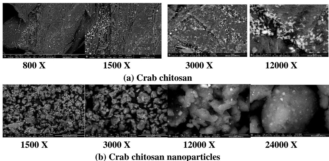
**Fig. 4.** SEM of (a) crab chitosan and (b) crab chitosan nanoparticles
