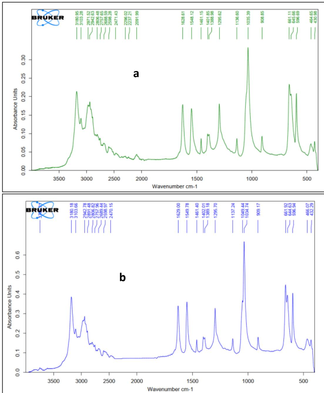
**Fig. 1.** FTIR of : (a) Crab chitosan and (b) Crab chitosan nanoparticles
