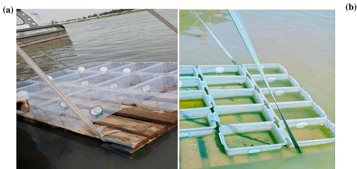
**Fig. 1.** Photos of *in situ* experiment showing samples collection: **(a)** Before filling out water in the enclosures, **(b)** during the treatment period.
