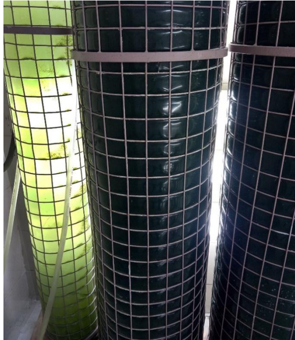
Fig. 1. The plastic vertical photobioreactors (200L) used as an inoculum for open pond cultivation
