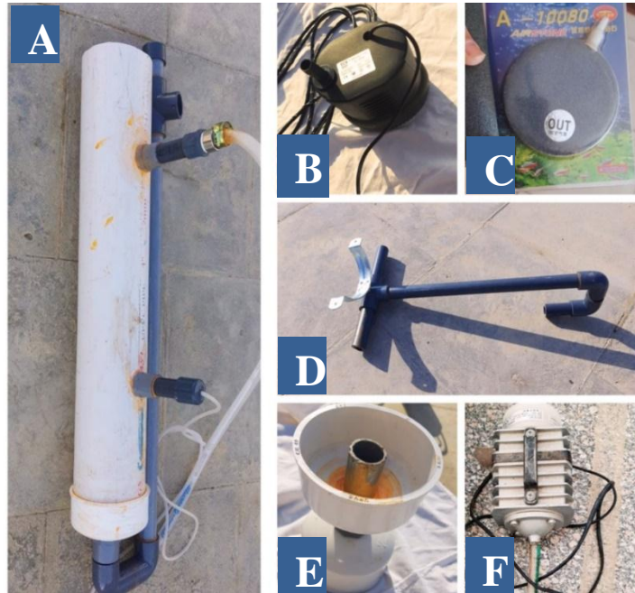
Fig. 3. The contents of the protein skimmer showing: (A): Protein skimmer body, (B): Water pump, (C): Air stone, (D): Device holder, (E): Foam cup and plug, and (F): Air pump
