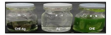
**Fig. 1.** The change in color using the *Cosmarium* hexane extract. Ag: silver nitrate solution, CHE: *Cosmarium* hexane extract, CHE-Ag (AgNPs): silver nanoparticles synthesized by *Cosmarium* hexane extract.
