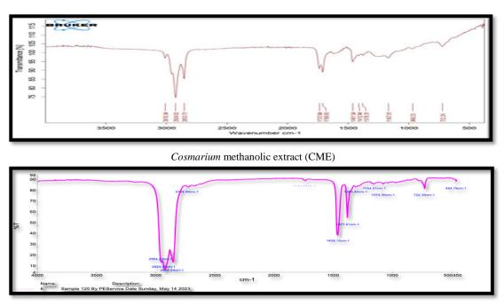
Fig. 6. FTIR spectra of Cosmarium-synthesized AgNPs
