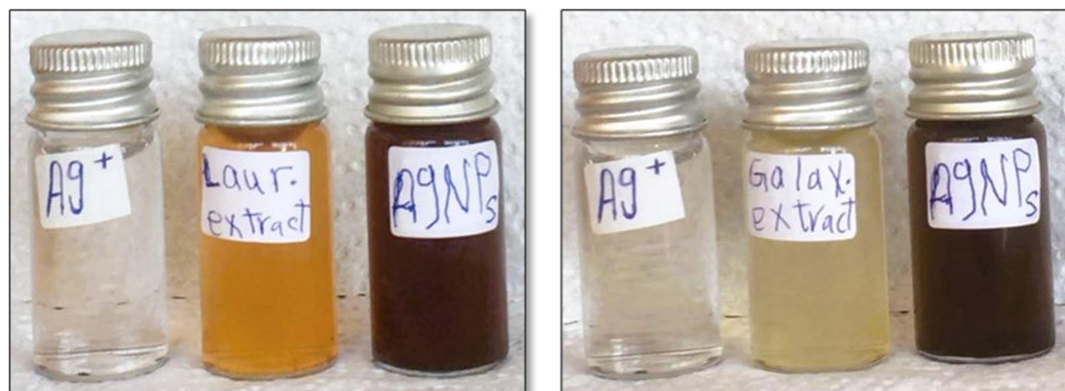
Fig. 3. Photo for the experiment showing the color change of both algal extracts; L. papillosa and G. rugosa on the addition of 10^{-3} M colorless solution of \text{AgNO}_3
