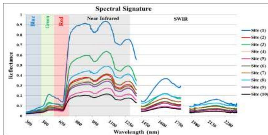
**Fig. 3: Hyperspectral signature values of mangroves at the ten sites measured at an average height of 40 cm above vegetation at nadir position**
