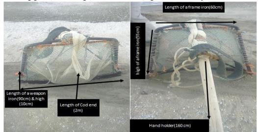
Fig. 2: Description of the fishing gear (hand dredge)
