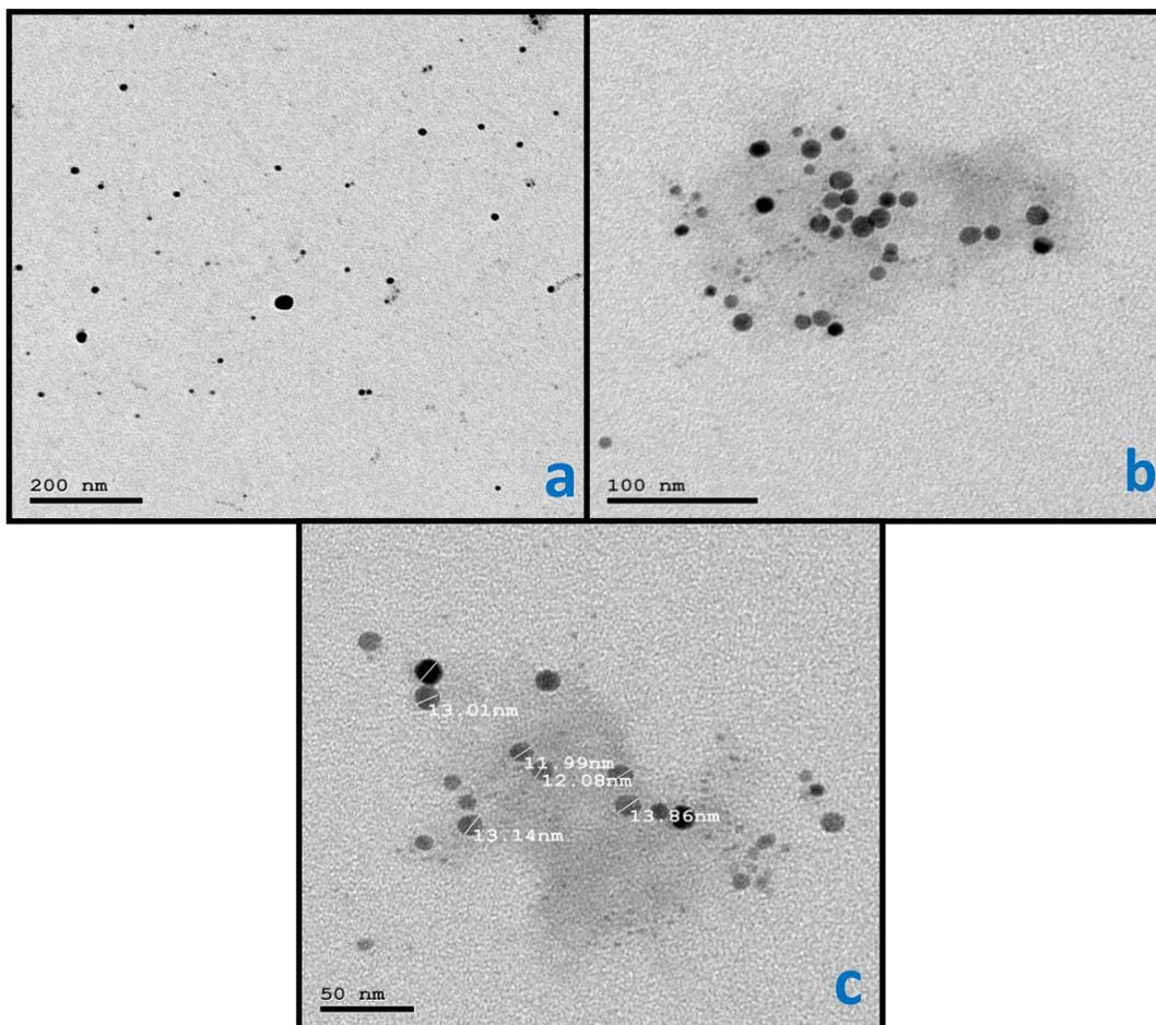
**Fig 3.** TEM images of MHB-AgNPs with scale bars of a) 200 nm, b) 100 nm and c) 50 nm
