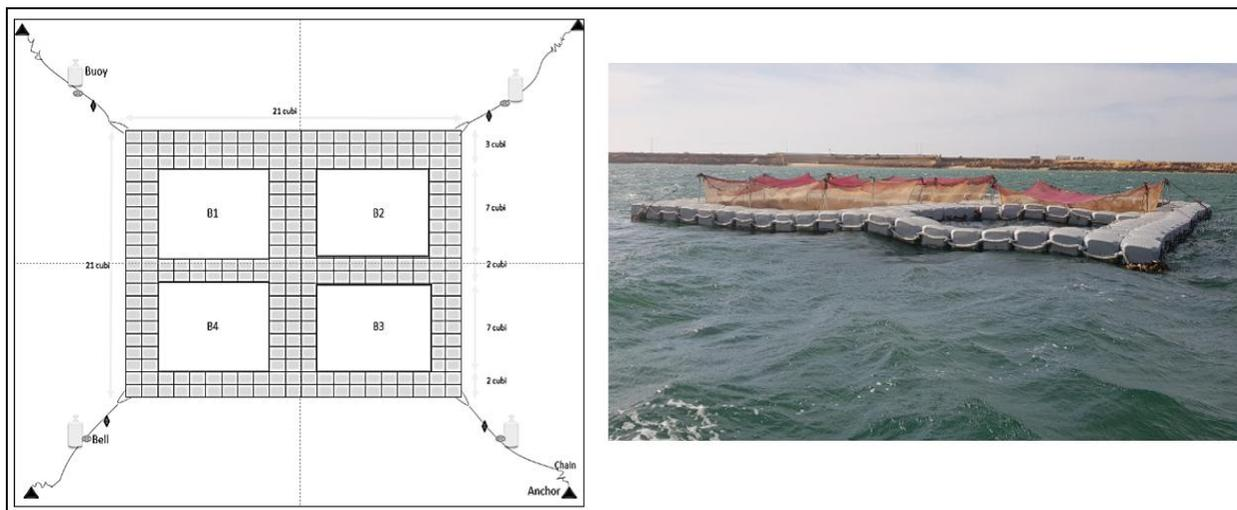
**Fig. 2 .** Basic components of the Cubi cage
