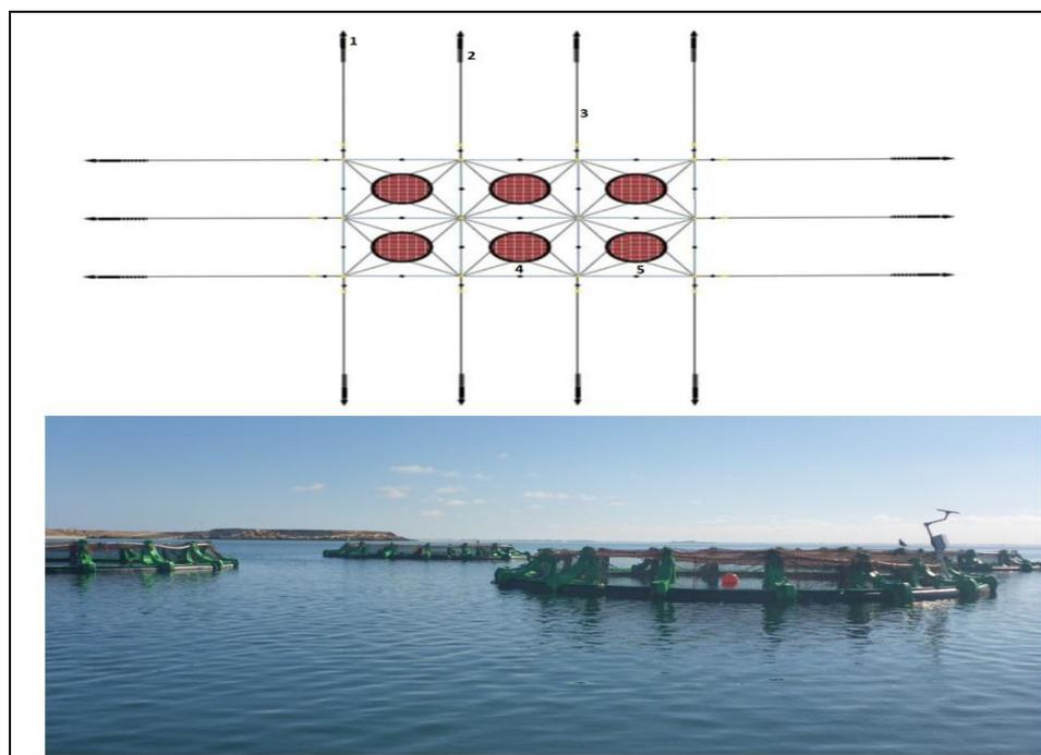
**Fig. 3.** Basic components of circular-shaped floating cages (1: Anchor, 2: Chain of 3m length, 3: Towing hawser of 40m length, 4: Cage containing 1 and 5 batches 5: Cage containing batch 2
