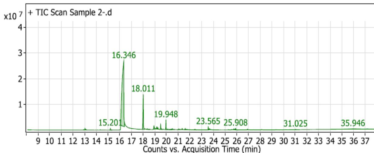
Fig. 4 Typical chromatograph of GC-MS with identified chemical from extract of ethyl acetate and diethylether of raw material of industrial incense.
