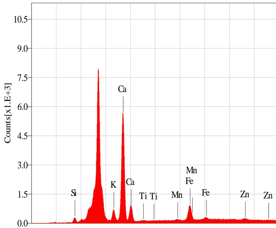
**Fig. 2** XRF material output of industrial incense.
