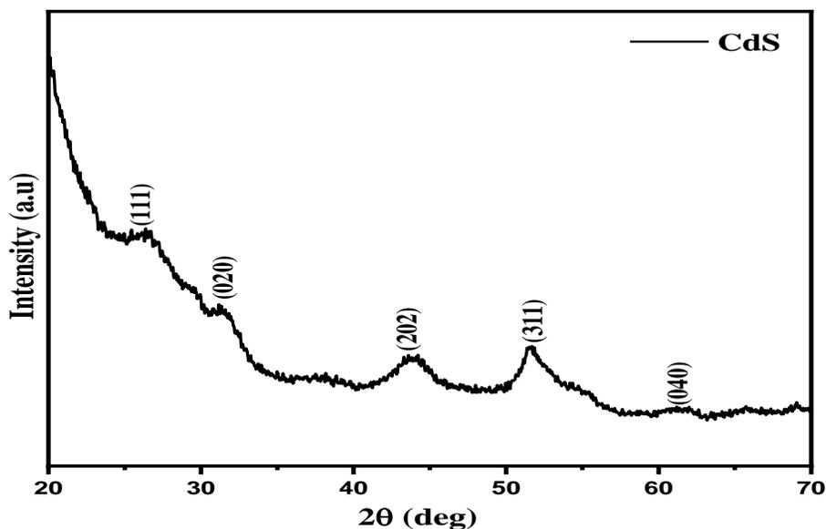
**Fig. 2** XRD pattern for CdS NPs
