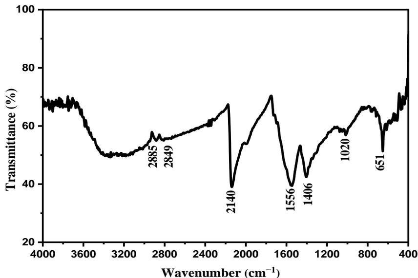
**Fig. 3** FTIR profile of green synthesized CdS NPs
