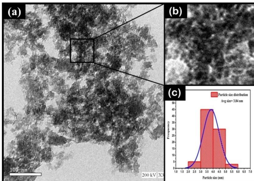
**Fig. 4** (a) HR\_TEM micrograph of green synthesized CdS NPs (b) Enlarged particle (c) Particle size distribution
