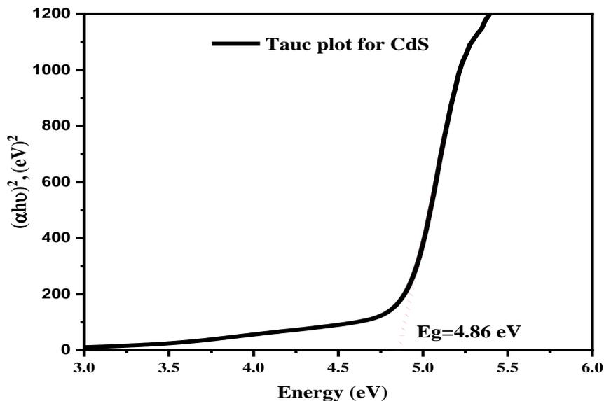
**Fig. 1b** The absorption coefficient vs. photon energy ( $h\nu$ ) for synthesized CdS NPs
