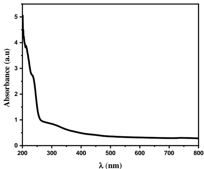
Fig. 1a. The absorbance spectra for synthesized CdS NPs.
