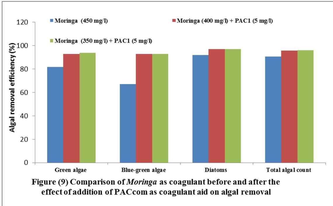
There is a triple effect of activated carbon addition, first, one is to minimize the coagulant dose, increase the efficiency of coagulation, and reduce disinfection by-products. (Kristiana et al., 2011) found that the removal of natural organic material improved by 70%, which led to a significant reduction (80-95%) in the formation of disinfection by-products.
