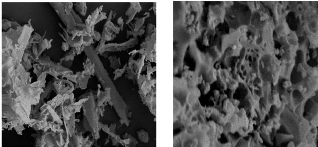
**Figure (11)** SEM micrographs of cotton stalks (left) and activated carbon produced from the activation of cotton stalks with KOH at 800°C (right).
