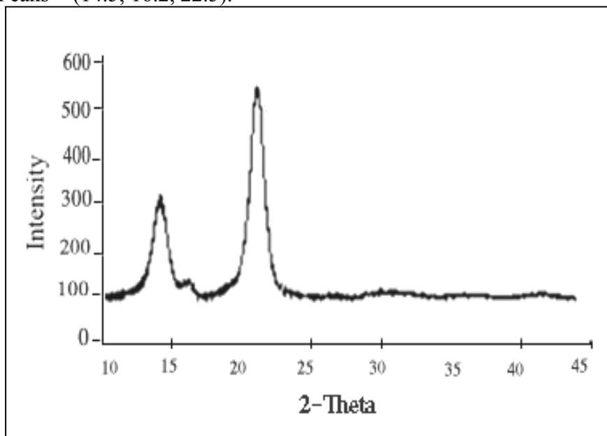
**Fig. 5.** X-ray patterns of the BC produced by *G. xylinus* during the current study on HSPO medium
