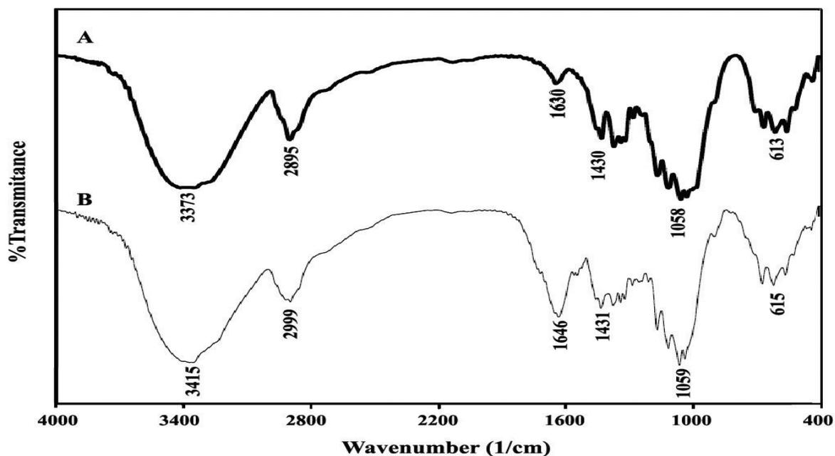
**Fig. 3.** FTIR spectra of the BC produced by *G. xylinus* during the current study (upper) standard BC (lower)
