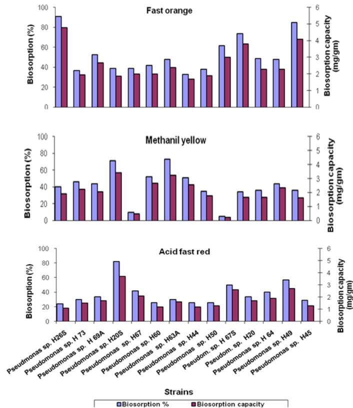
Fig. 3. Decolorization percentage and biosorption efficiency of dye removal by *Pseudomonas* strains.
