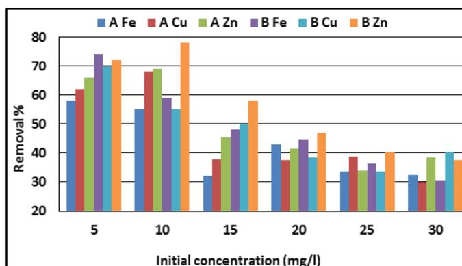
Fig. 10: Effect of initial concentration on removal percent of heavy metals from wastewater using (A: chitosan) and (B: activated carbon).
