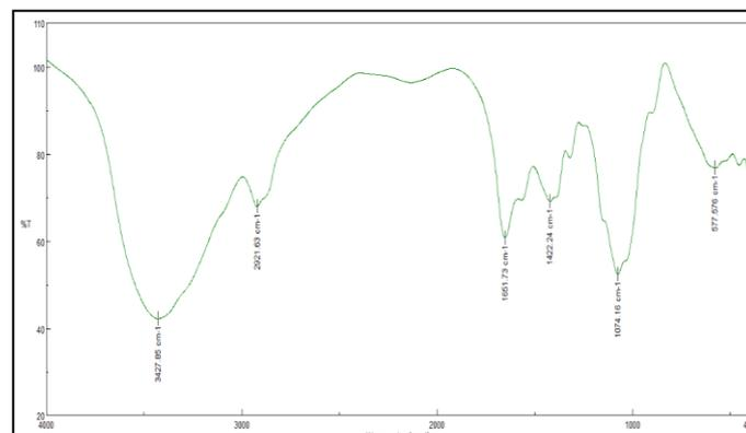
Fig. 3: FTIR spectrum of activated carbon
