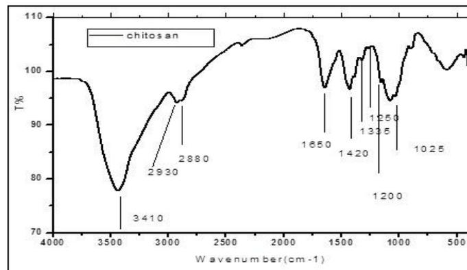
Fig. 2: FTIR spectrum of chitosan
