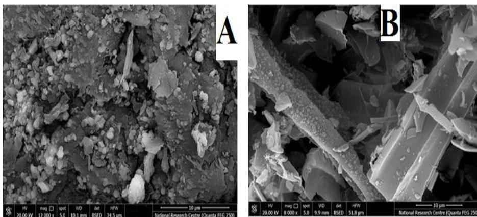
Fig. 1: SEM image of (A) chitosan and (B) activated carbon.
