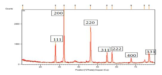
**Fig. 13.** X-ray diffraction of the nanoparticles fabricated from the extract of *E*. *intestinalis*
