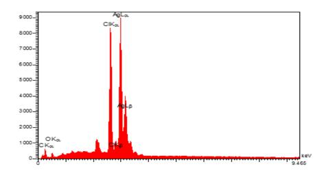
**Fig. 11.** Energy-dispersive X-ray spectroscopy analysis of the synthesized silver nanoparticles from the extract *E. intestinalis*
