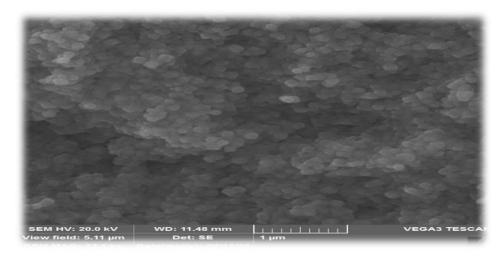
**Fig. 12.** Scanning electron microscope image of the nanoparticles fabricated from the extract of *E. intestinalis*
