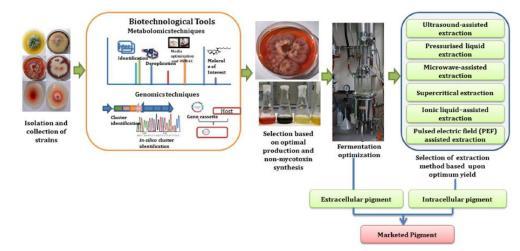
Fig. 2. Schematic roadmap for a pigment journey from lab scale to industrial
