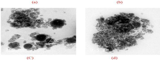
**Fig. 1.** TEM image (**a**,**b**) showing ZnO nanoparticles (ZnONPs) with size ranging from 5-15nm in diameter, and TEM image (**c**,**d**) showing selenium nanoparticles (SeNPs) of size ranging from 20-40nm in diameter.
