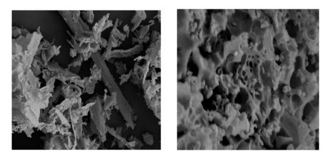
Figure (11) SEM micrographs of cotton stalks (left) and activated carbon produced from the activation of cotton stalks with KOH at 800°C (right).
