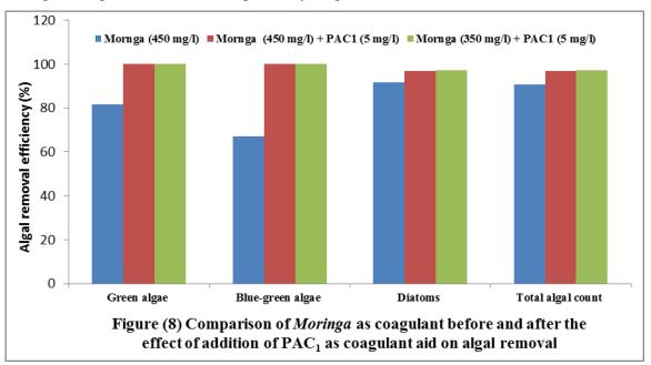
Also, the result revealed that with the addition of different doses of *Moringa* seed extract (450, 400, 350, 300, 250 mg / l) to the commercial activated carbon dose (5 mg / l), the
